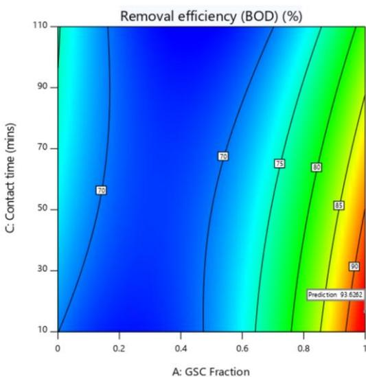
(a) **Figure 5:** 3D surface plot (a) and the corresponding contour plot (b) for the effect of interaction of contact time and groundnut shell char fraction on BOD removal efficiency
