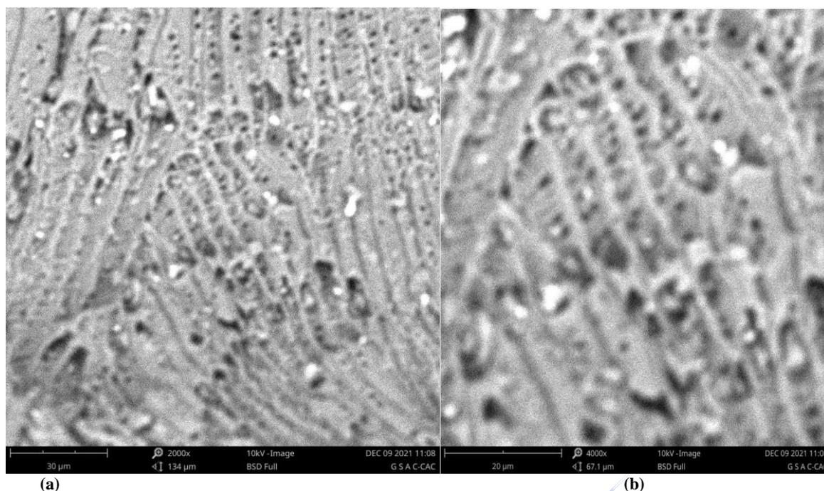
**Figure 3: SEM micrograph of composite activated carbon**
