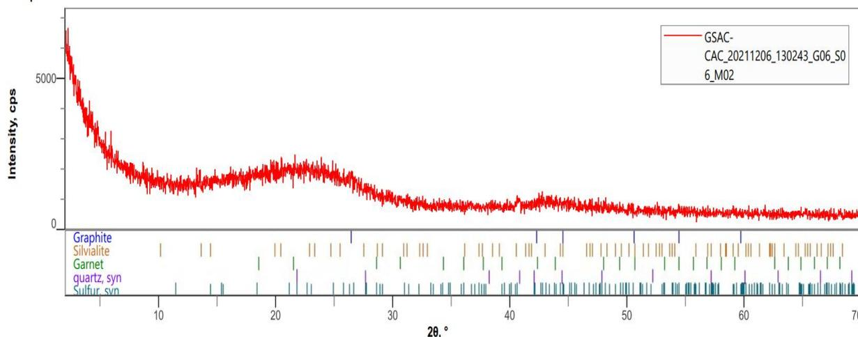
**Figure 2: XRD spectra of composite activated carbon**
