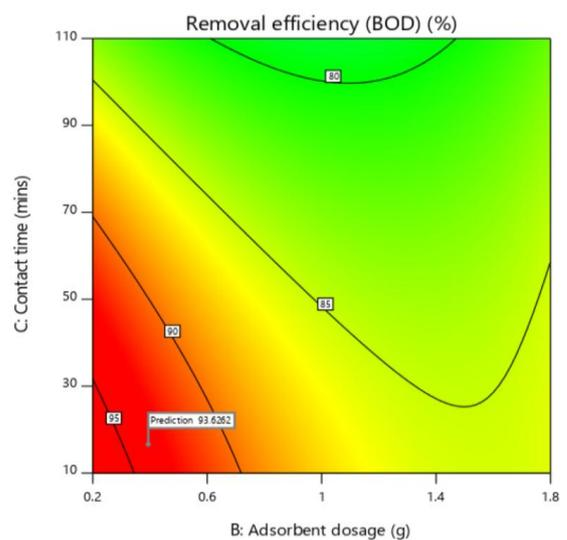
(b) **Figure 6:** 3D surface plot (a) and the corresponding contour plot (b) for the effect of contact time and adsorbent dosage on BOD removal efficiency
