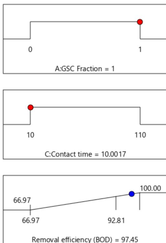
**Figure 7:** Desirability ramp showing optimal conditions of BOD uptake in pharmaceutical wastewater
