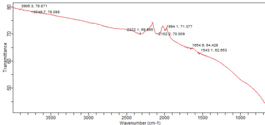
**Figure 1: FTIR spectra of composite activated carbon**
